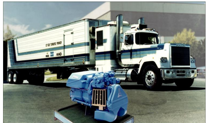
1980 – Mack Superliner truck with a GT601 vehicle gas turbine drive unit
