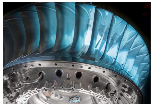
Additively manufactured bearing housing (diameter 1,5m) with generatively manufactured blades
