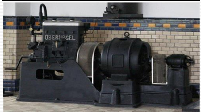
Motor model 35 (LM116) in the factory museum and as a generator drive in the old waterworks in Hattersheim
