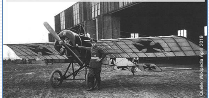
Pfalz E.1 with a rotary engine from Oberursel.
