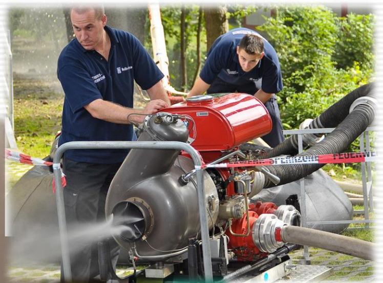
Picture above: T216 portable pump in use with the company fire brigade.
