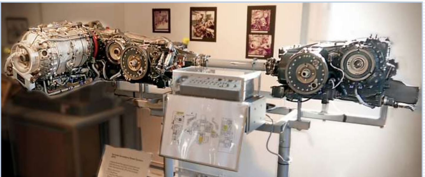
The functional model of the Secondary Power System Tornado in the factory museum
