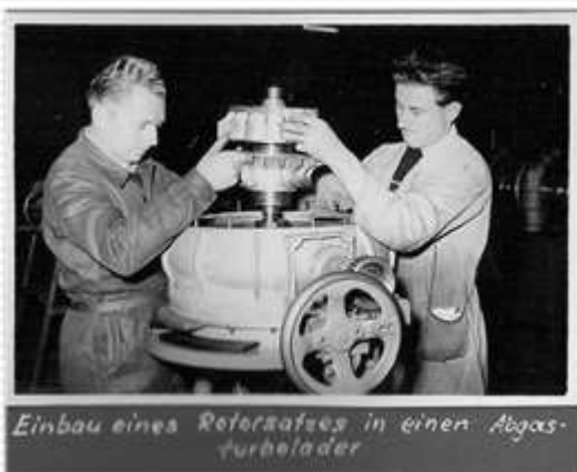
Installation of a rotor assembly into an exhaust gas turbo charger.
