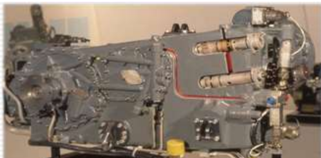
Clearly visible: the cast-in channels
